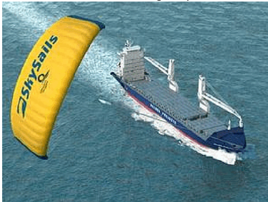
Figure 9. SkySails Concept Applied to Commercial Cargo Ship
