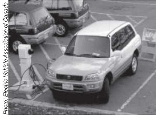
Photo: Electric Vehicle Association of Canada Toyota's RAV4-EV (shown above) is one of several battery-electric vehicles that have been manufactured by major automakers over the last decade.
