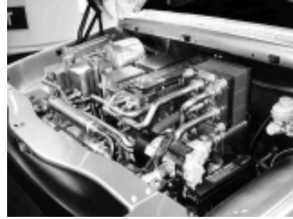
Fuel cell system in the Chrysler FCEV fuel-cell vehicle.
